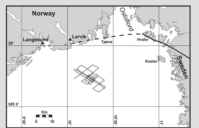
Drawn black line/stippled line represents the location of the Hvaler/Tjøme/Trollhättan ice marginal zone, dated to 13 400-14 200 cal y BP (ref. 4, 12). The track lines of the chirp sonar profiles are also shown. The coring site of MD99-2286 was deglaciated sometimes between 14 500 and 13 600 cal y BP. Redrawn from ref. 12.
