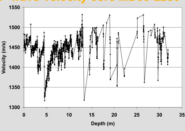
P-wave velocity in core MD99-2286, measured with 0.5-cm resolution using MSCL. The acoustic signal was lost due to insufficient coupling in the interval 10.8 11.7 m, and in virtually all measurements below 13 m. Abrupt changes in the core top are artefacts.
