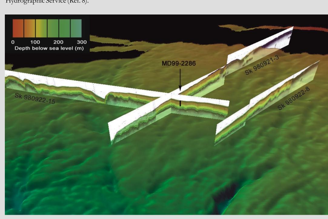
Oblique view of multibeam bathymetry and chirp sonar profiles around the coring location of MD99-2286. The chirp profile names are indicated, and the core MD99-2286 is marked with a black bar below the arrow. The bathymetric terrain model is made partly transparent in order to make the chirp profiles visible. Colours on the chirp profiles mark interpreted seismic units. Multibeam bathymetry from Norwegian Hydrographic Service (ref. 8).
