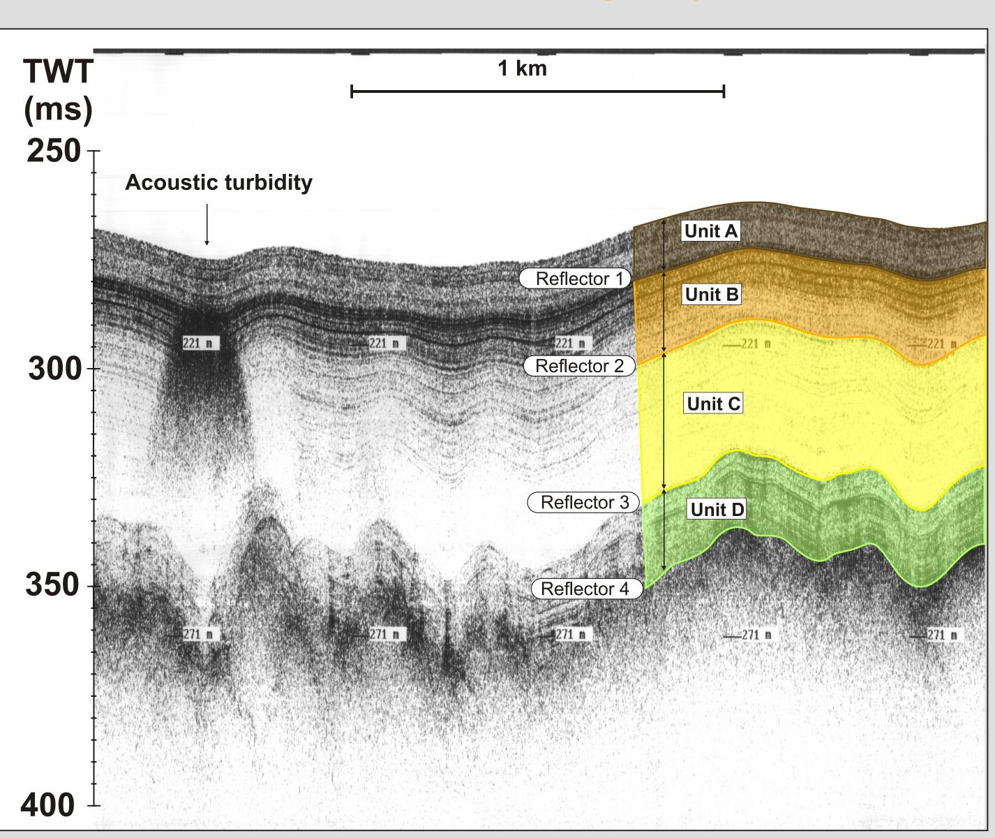
Chirp record showing the general stratigraphy of the survey area in northeastern Skagerrak. The defined seismic reflectors 1-4 and units A-D are indicated. A small patch of acoustic turbidity is marked with an arrow. Depth labels indicate approximate depth from the tow-fish in metres based on a sound velocity of 1500 m/s. Average towing depth for the chirp sonar tow-fish was ca 15 m below sea level. Chirp section located at N58°43.9', E10°14.6'.
