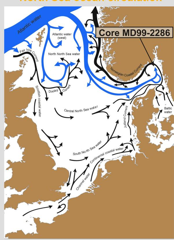
General circulation pattern in the North Sea and Skagerrak. The relative magnitude of volume transport is indicated by the width of the arrows. Blue arrows indicate water entering the Skagerrak more or less directly from the Atlantic and black arrows indicate indirect transport via the North Sea (redrawn from ref. 4).
