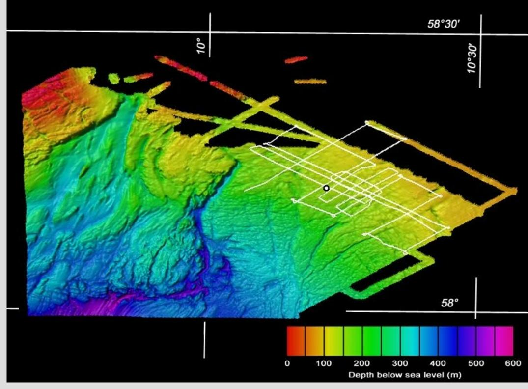
Three-dimensional shadow relief model of bathymetry in northeastern Skagerrak. Chirp sonar profiles are shown as white lines, and core MD99-2286 is indicated with a circle. Multibeam bathymetry data from the Norwegian Hydrographic Service (Ref. 8).
